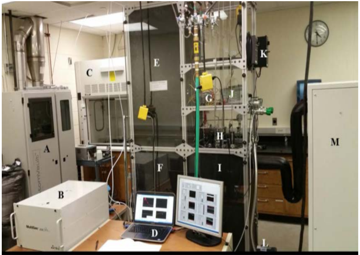
Figure 5-2. Natural gas capable apparatus with cylinder gas cabinet (A), Sample analyzer (B), exhaust fume hood for flaring and venting (C), computer control interface (D), bubbler and separator cold box (E), reservoir cold box (F), data acquisition (G), mass flow controllers (H), heat exchange and pumping cold box (I), mass flow controller power supply (J), pump motor controller (K), pump motor (L), cryocooler (M)
